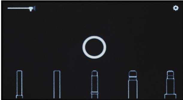
The five drawings on the bottom of the screen represent the five different types of fittings which are supported by the corresponding light sources at the front of the device. If you are uncertain which source matches your fitting, you can press the image on the screen and a photograph of the actual fitting will be shown.
