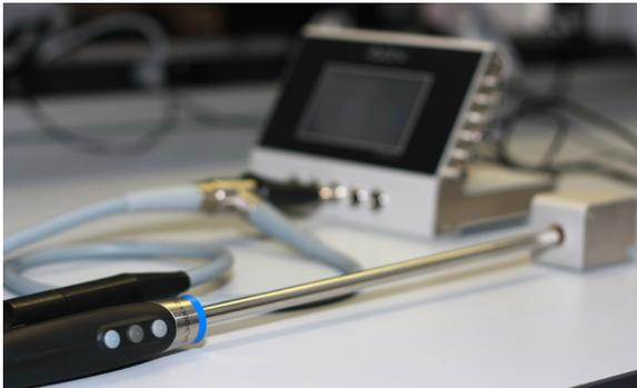
After the EndoEye feature has been installed on your LG20-e, the main screen shows an additional icon, next to the Endoscope test mode icon, to access the EndoEye test mode.
